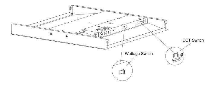
The end users may adjust the color temperature and lumen output respectively by the two DIP switch. Each DIP switch is accommodated with 3 options (left, middle and right), corresponding to 3 color temperatures and 3 powers respectively, which can perform the desired color temperature and lumen output combination.
